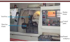
Fig 1 Photographic view of CNC Lathe machine
